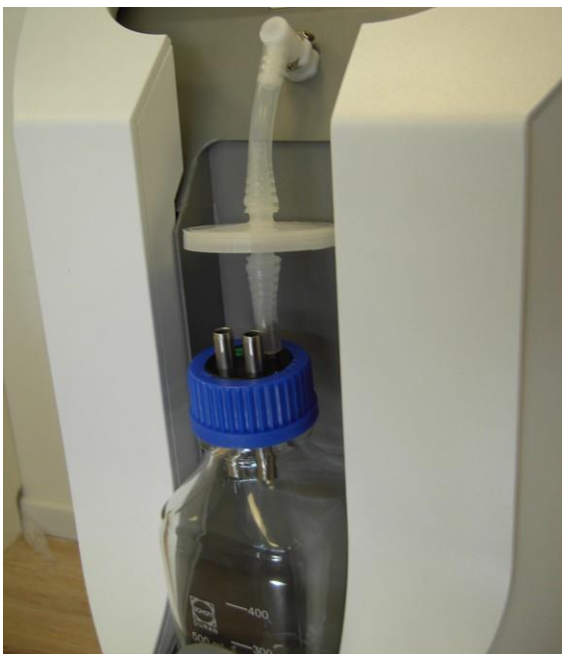
Figure 3-44. Ensemble de filtre installé
